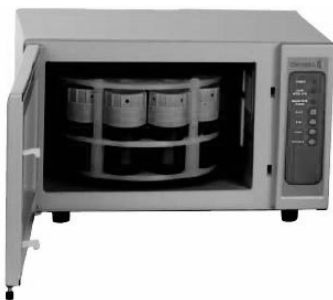
Fig. 2 Front view of microwave digester system
